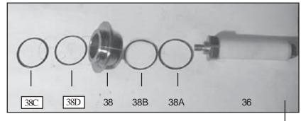
10. If o-rings (38A and 38C) or support rings (38B and 38D) are damaged, replace with new parts. Examine plunger (36) for wear.
